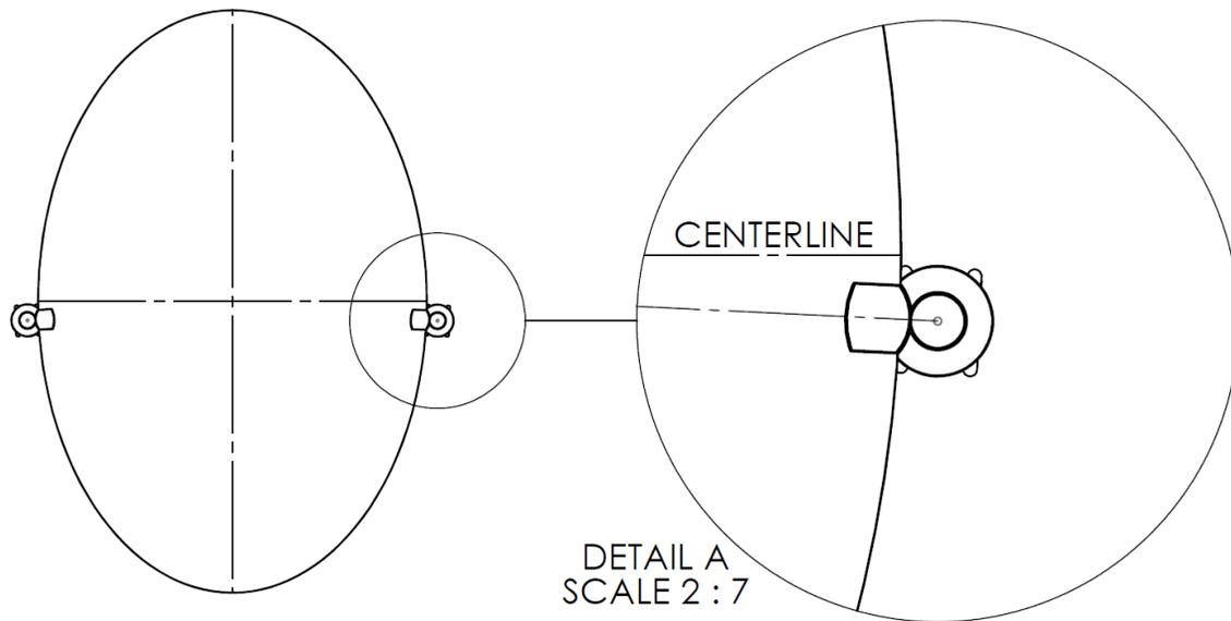
For oval and round mirrors, it is advised that the mounting post assemblies be installed slightly below center, at a perpendicular angle to the tangent line. This provides the mirror assembly with extra support.
